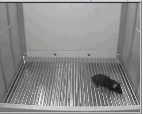
**4) Lighting.** The absolute lighting level is not critical, as long as there is **enough light** in the chamber to give a clear image on the screen. If you do not have a auto-iris lens (one with a short wire that plugs into the camera), adjust the aperture manually so that a clear image is visible on the screen.
